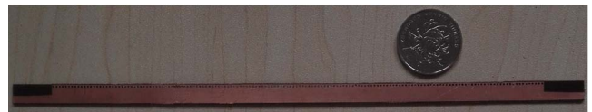
Fig. 9. Photography of the fabricated HMSIW leaky-wave antenna and the parameters and coordinate correspond to the ones in Fig. 6. L_s = 188.4 mm, w_2 = 0.2 mm, w_1 = 6.3 mm, S = 1.2 mm, and the diameter of via is 0.7 mm.
